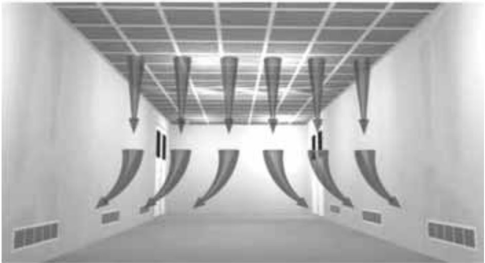
Figure 7 Unidirectional displacement of dirty air
