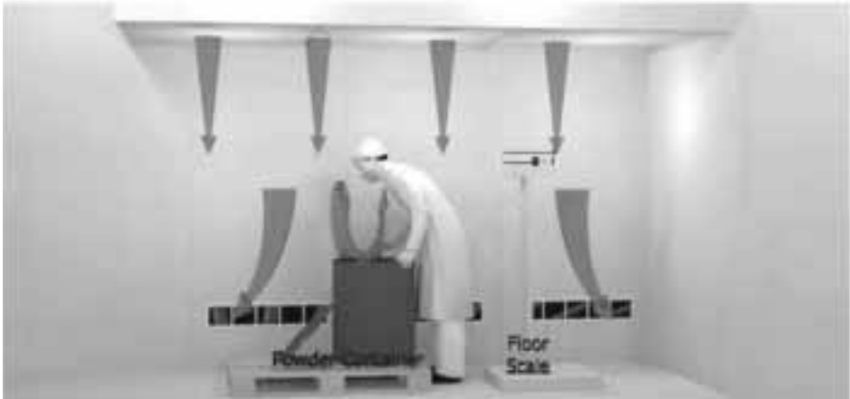
Figure 15 Operator subject to powder contamination due to airflow reversal in bin
