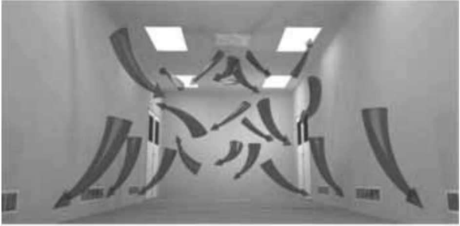
Figure 6 Turbulent dilution of dirty air
