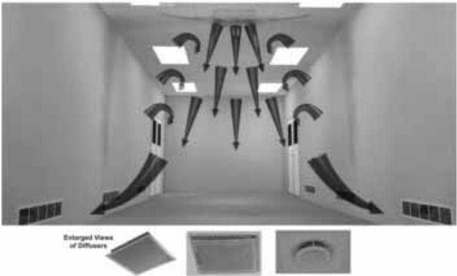
Figure 10 Perforated plate diffuser
